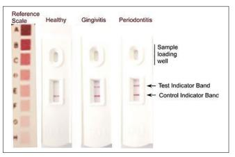
$\ensuremath{\textit{Fig. 2}}$   $% \ensuremath{\textit{Analysis}}$  of salivary samples by lateral flow assay and representative image.
