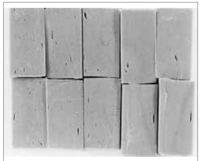
Fig. 1 Ten sliced specimens of an impression sample of group 1 (Permadyne HV, "stropping technique"). A considerable amount of voids is visible.
