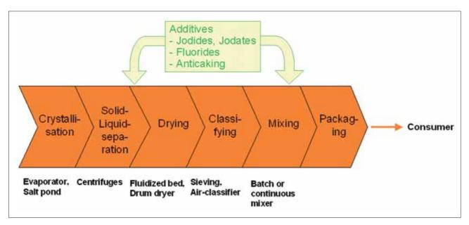
Fig. 1 Typical process chain during the production of salt with additives
