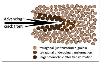
**Fig. 1 "Transformation toughening"** of an advancing crack in a block of stabilized zirconia. The phase transformation of the zirconia crystals from tetragonal to monoclinic with the associated volume expansion can put the crack into compression, retarding its growth and enhancing the fracture toughness of the material.
